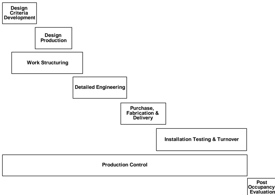
In the first phase, which begins in design production and work structuring, decisions about the selection of materials, their joining, and configuration on site constrain the work method. For example, the choice of tilt up panels over masonry limits downstream choices about the work method. We have been tinkering with the idea that the first phase can be understood as a funnel where the surface of the funnel are the time, cost and quality boundaries. The
